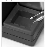
Use the slots to remove remaining particles.
